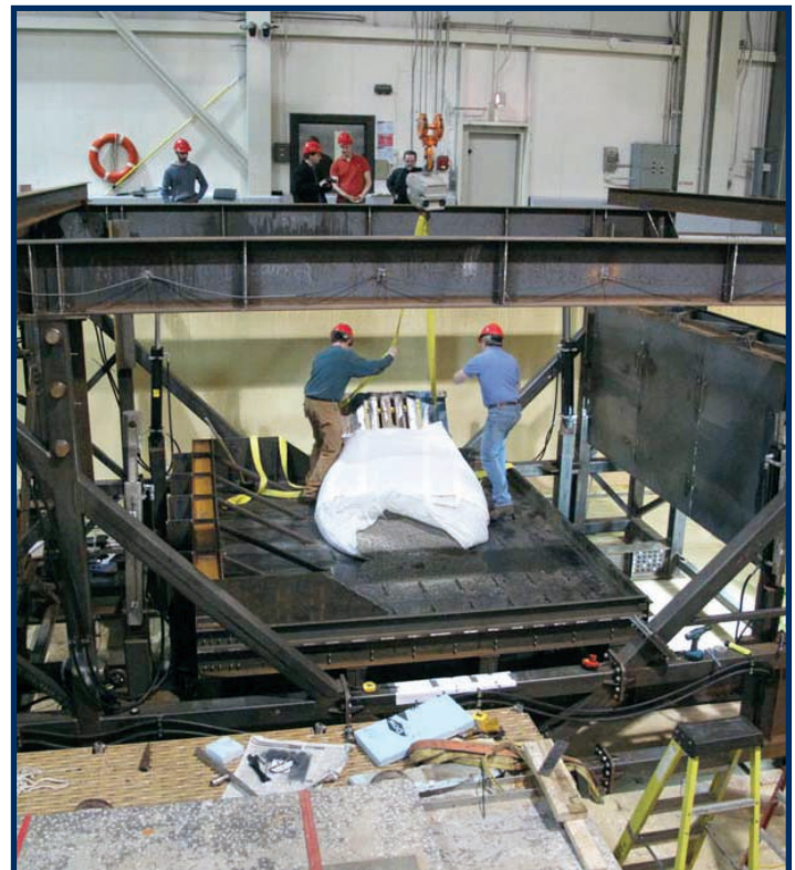
Test frame in ice tank prior to filling
