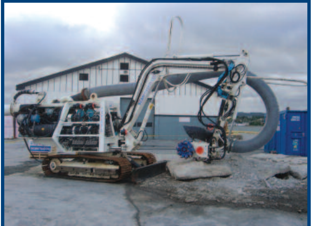
Pro-Dive Scanmudring Sub Sea Excavator With New Cutting Unit
